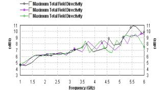
**Fig: 3.** Antenna Directivity Comparison Curve for Base Shape, Single Slotted Patch and Five Slotted Patch
