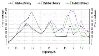
**Fig: 4.** Antenna Efficiency Comparison Curve for Base Shape, Single Slotted Patch and Five Slotted Patch
