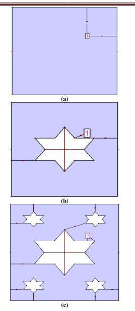
**Fig: 1:** Antenna Layout (a) Base shape (b) Single slotted shape (c) Five slotted shape
